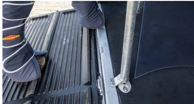
Optimum foothold and minimised risk of slipping due to safety treads, side stops on the rear ramp covering and the narrow rear ramp hinge.
