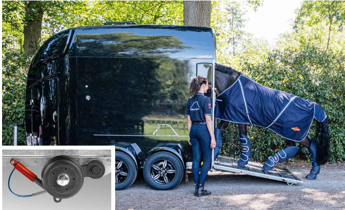
Low loading height due to the lowered "CFFplus" comfort suspension chassis with wheel shock absorbers and soft suspension.
