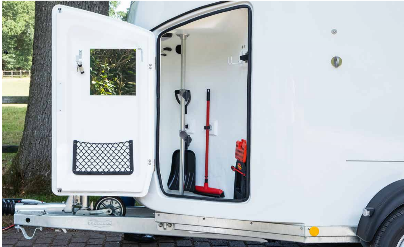
Convenient operation and extensive standard features in the tack locker with a door catch as well as a telescopic broom, plastic shovel, door net, mirror, crop holder, large bridle hooks, pad holder, LED light and folding stool with safety catch.
