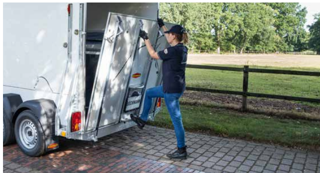
Robust rear ramp with four galvanised steel profile struts with integrated lifting device; additionally with new, robust double step.
