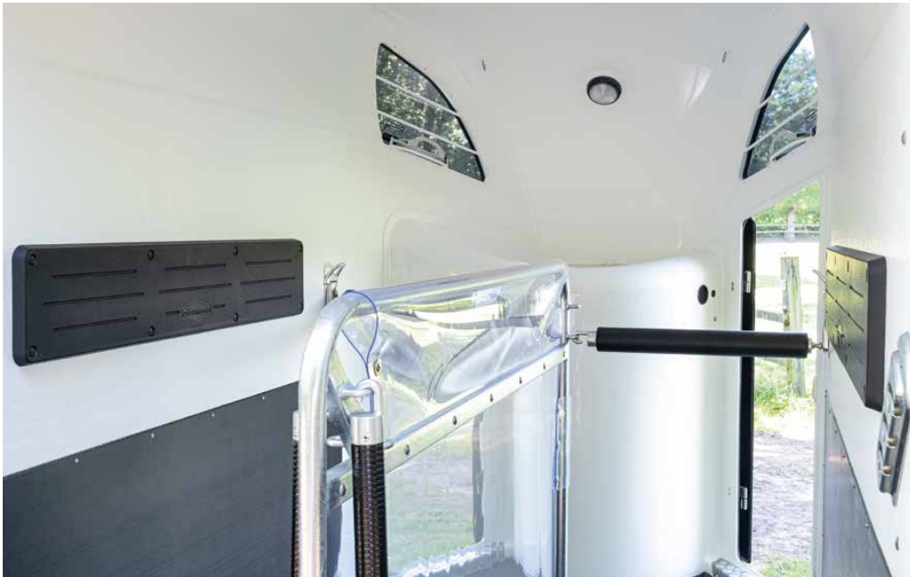
Safe transport ensured by the track-proven Böckmann partition wall system and the safety stall bar system (MSS) with tie rings and an adjustable height range of 10 cm. Further protection is provided by the additional stall bar padding as well as the padding and kick protection on the side walls (the latter is an accessory).
