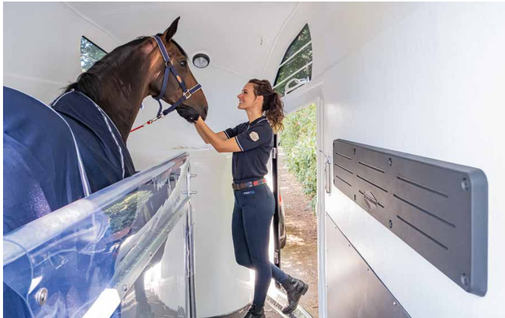
Safe transport ensured by the track-proven Böckmann partition wall system and the safety stall bar system (MSS) with tie rings and an adjustable height range of 10 cm. Further protection is provided by the additional stall bar padding as well as the padding and kick protection on the side walls (the latter is an accessory).
