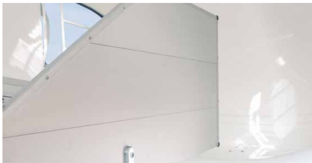
Safe transport due to the aluminium head divider wall e.g. for transporting two stallions.
