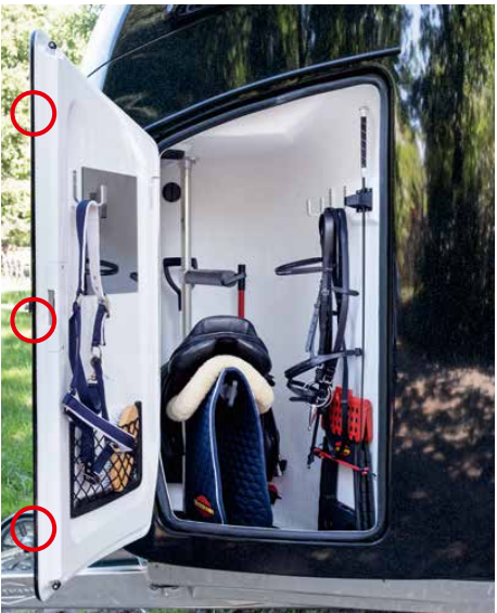
Everything is conveniently accessible from outside with the large tack locker door with rain gutter. Perfect closure with the 3-point door lock and rubber seal.
