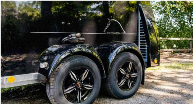
Mudguards as shelf with the wide and open, straight form of the impact-resistant plastic or polyester mudguards (accessory).
