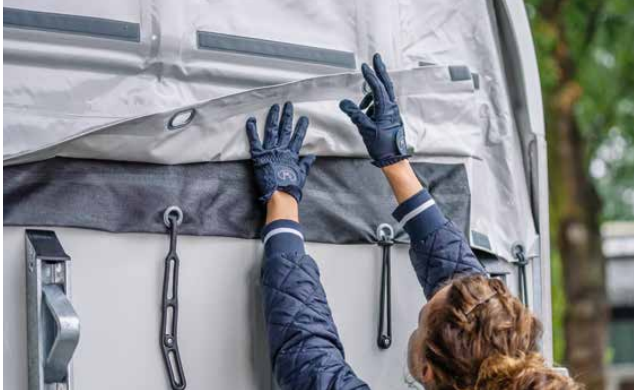
PVC canvas lift with integrated net and roll-up function.
