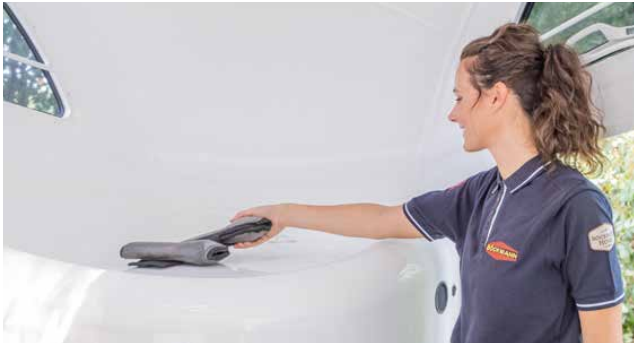
Tack locker as a shelf with an optimised design and plenty of space and no biting edge for the horses. Practical cleaning with defined water drainage.
