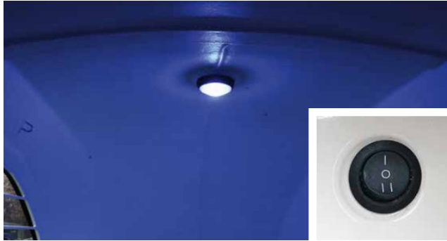
Calming atmosphere provided by the blue LED transport light – can be conveniently switched from blue to white.
