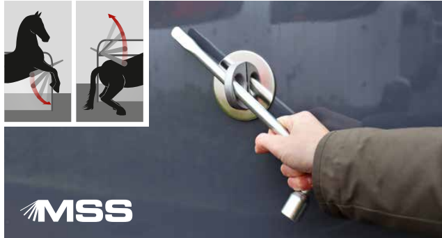
Fast safety in the event of an emergency with the track-proven Multi Safe safety stall bar panic system (MSS). Can be released at the front and rear. The wheel spanner is included in the standard equipment.
