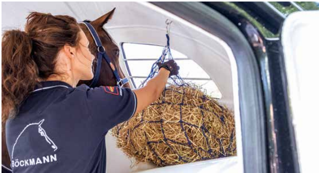
Easily accessible hay with optimally positioned hooks and counterholder for a hay net. The specially shaped tack locker with its large radii does not have any biting edges for the horse.
