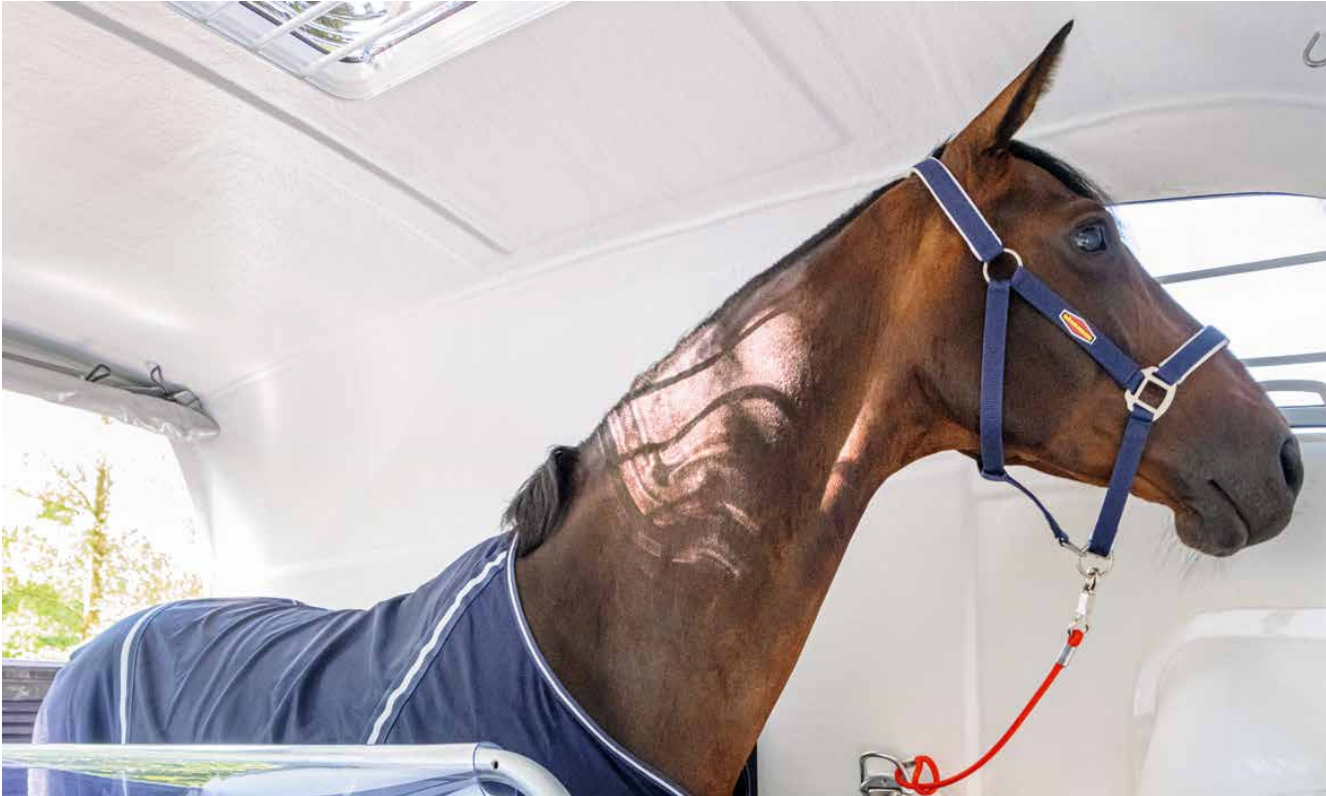
Plenty of headroom, space and light interior due to the generous space concept of the Comfort model. The tinted pop-up windows with integrated grille, large radii without corners and edges and flat hinges provide additional protection.
