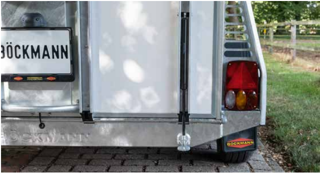
No slipping of the horse's hooves and good visibility from the car due to closed, perforated rear struts; the large lighting unit is visible even when the rear ramp is open.
