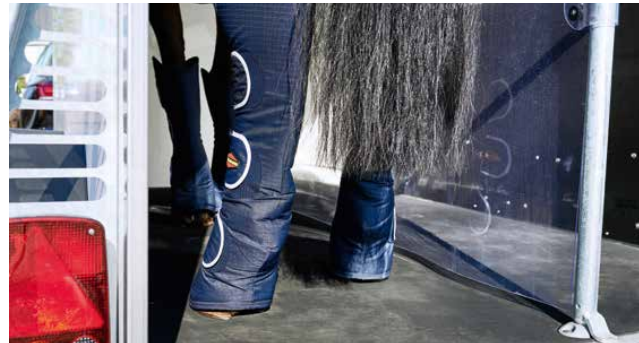
Lots of room for a wide stance due to securing of the PVC curtain 600mm above the floor – for comfortable transport.
