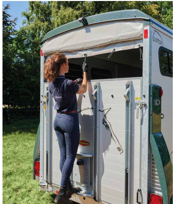
Robust rear ramp with four galvanised steel profile struts with integrated lifting device for easy opening of the rear ramp, additionally with new double step.
