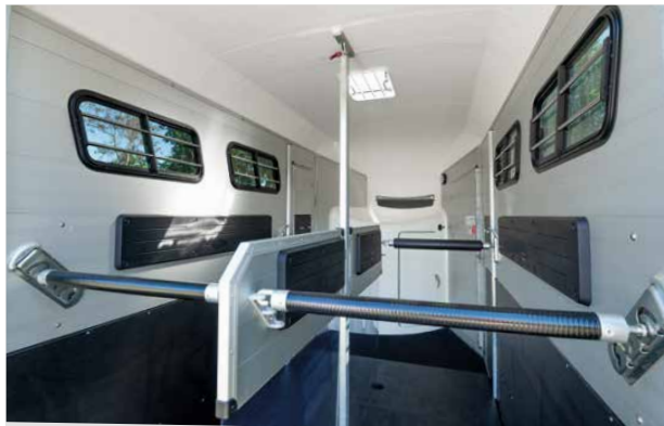
Safe transport is ensured by the track-proven Böckmann partition wall system and the safety stall bar system (MSS) with tie rings and an adjustable height range of 10 cm. Further protection is provided by the additional stall bar padding as well as the padding and kick protection on the side walls.
