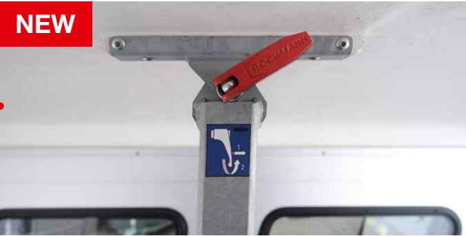
Eccentric clamp for easy removal of the centre post partition wall, for example when transporting a mare and her foal.
