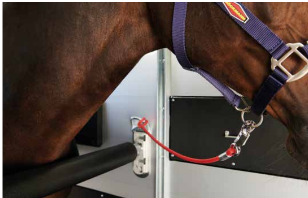
Safe transport is ensured by the track-proven Böckmann partition wall system and the safety stall bar system (MSS) with tie rings and an adjustable height range of 10 cm. Further protection is provided by the additional stall bar padding as well as the padding and kick protection on the side walls.
