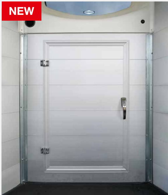
Alu cabinet in front available as an accessory instead of the standard tack locker for the Portax E and L E. The anodised aluminium body with large entrance door securely separates the horse compartment from the full polyester bow and allows use of the interior space behind. Telescopic broom, plastic shovel, riding crop holder and door nets are part of the standard equipment.
