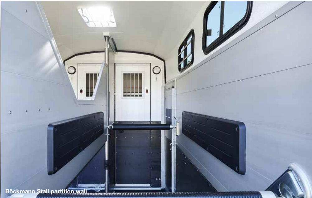
Safe transport is ensured by the track-proven Böckmann partition wall system and the safety stall bar system (MSS) with tie rings and an adjustable height range of 10cm. Further protection is provided by the additional stall bar padding as well as the padding and kick protection on the side walls and on the tack locker in front of the horses (the latter is available as an accessory for the Portax SKA and L SKA). Also refer to page 54.
