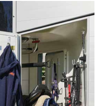
Protection from rain by the rain guttering above the tack locker door.
