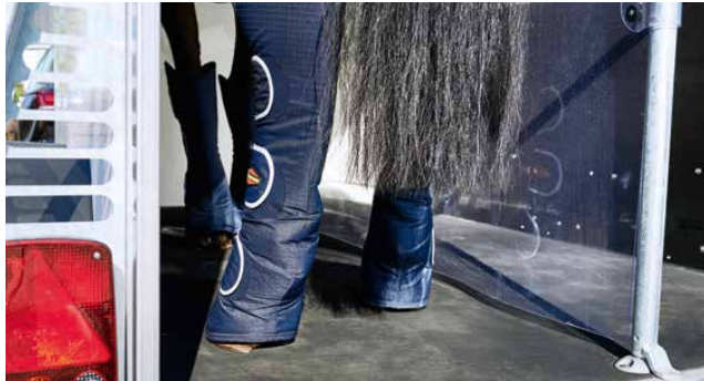
Lots of room for a wide stance due to securing of the PVC curtain 600mm above the floor – for comfortable transport (Böckmann partition wall is an optional accessory).
