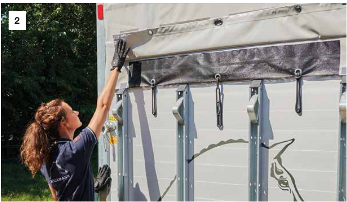
Canvas lift with automatic roll-up function (Big Portax) [1] and integrated net (Portax and Portax L) [2].
