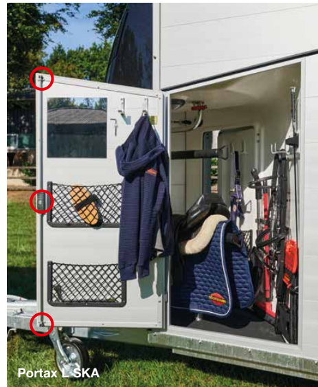
Optimum closure with the 3-point door lock and rubber seal.
