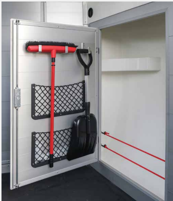
Alu cabinet in front available as an accessory instead of the standard tack locker for the Portax E and L E. The anodised aluminium body with large entrance door securely separates the horse compartment from the full polyester bow and allows use of the interior space behind. Telescopic broom, plastic shovel, riding crop holder and door nets are part of the standard equipment.
