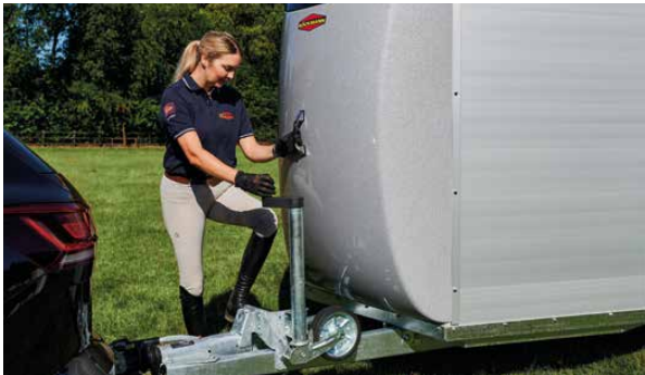
Simple operation due to the automatic jockey wheel, extra-long with handy plastic crank, perfect to operate even in cold weather (heavy duty jockey wheel on the Big Portax models).
