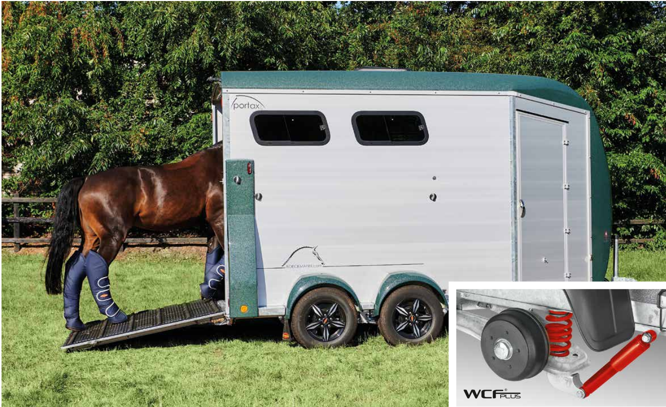
Low loading height with the lowered World-Class chassis (WCF) with galvanised independent wheel suspension, coil spring suspension and wheel shock absorbers.
