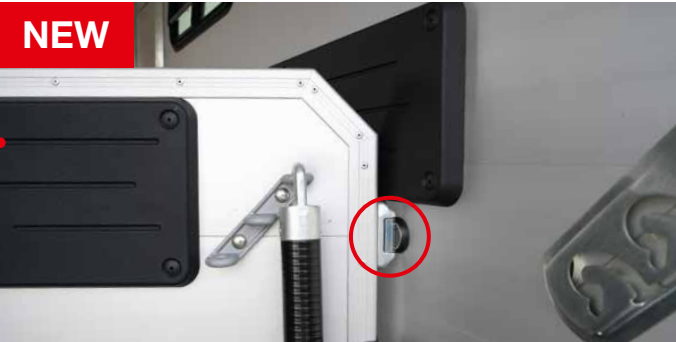
Simple fixing of the partition wall sections on both sides using practical magnetic stops for even more convenience during loading.
