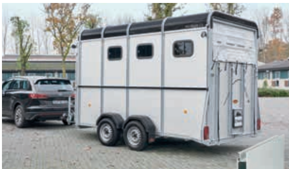
Robust structure made of anodised aluminium double web profile for safety and durability.
