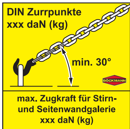
Fig. 5: Lashing points on the trailer
