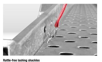
With four lashing shackles to secure your load during transport. All lashing shackles can be lowered into the loading area by means of a spring.
