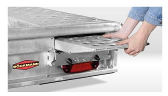
Drive-on rails can be slid underneath
