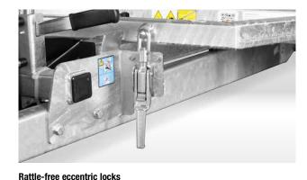
to secure the upper bridge. Easily accessible due to the new positioning at the front of the trailer.
