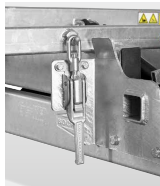
Rattle-free eccentric locks to secure the upper bridge. Easily accessible due to the new positioning at the front of the trailer.
