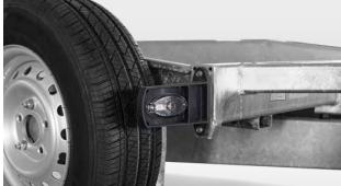
Optimally positioned LED clearance and marker lights to keep in view the maximum vehicle width from the towing vehicle. Rear lights optionally also available as LED lighting.
