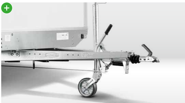
Solid automatic jockey wheel for safe stability and fast cranking.
