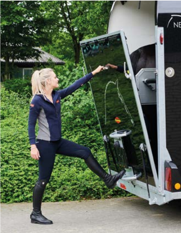
Robust rear ramp with integrated lifting device; additionally with robust double step.
