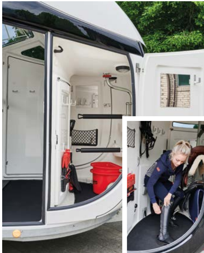
Convenient operation and extensive standard features in the tack locker and tack room with a door catch as well as a telescopic broom, plastic shovel, door net, mirror, crop holder, feed troughs, large bridle hooks, pad holder, LED light and folding stool with safety catch.
